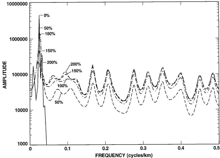
FIG. 4. Burg spectra for sine waves with average white noise contributions of 0 through 200%. After adding the white noise, each data set was normalized to a standard deviation of 1 prior to calculating its Burg spectrum. As the amount of white noise increases the main peak amplitude decreases.
