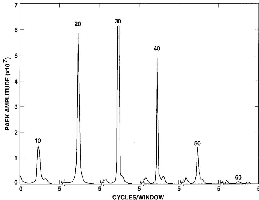
FIG. 3. Sine wave power spectra for prediction error filter orders of 10, 20, 30, 40, 50, and 60. Power spectra are generated for a simple sine wave using a data window of 100 points and a variety of filter orders. The maximum spectral peak occurs for a filter order of 30.
